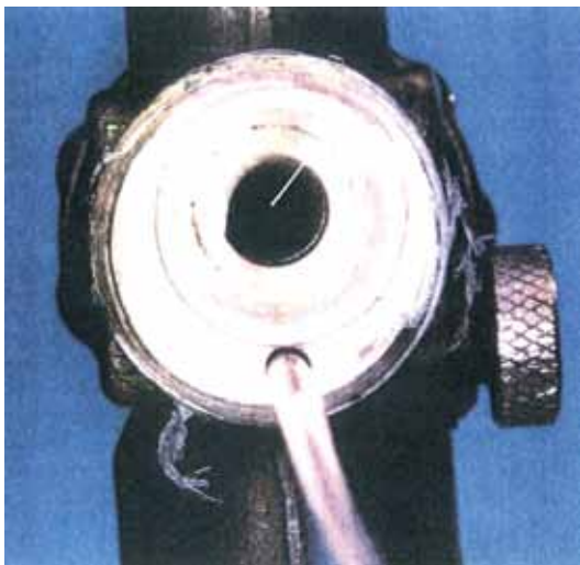
Figure 19 – The witness marks (arrow) left by the missing excess flow valve spring
